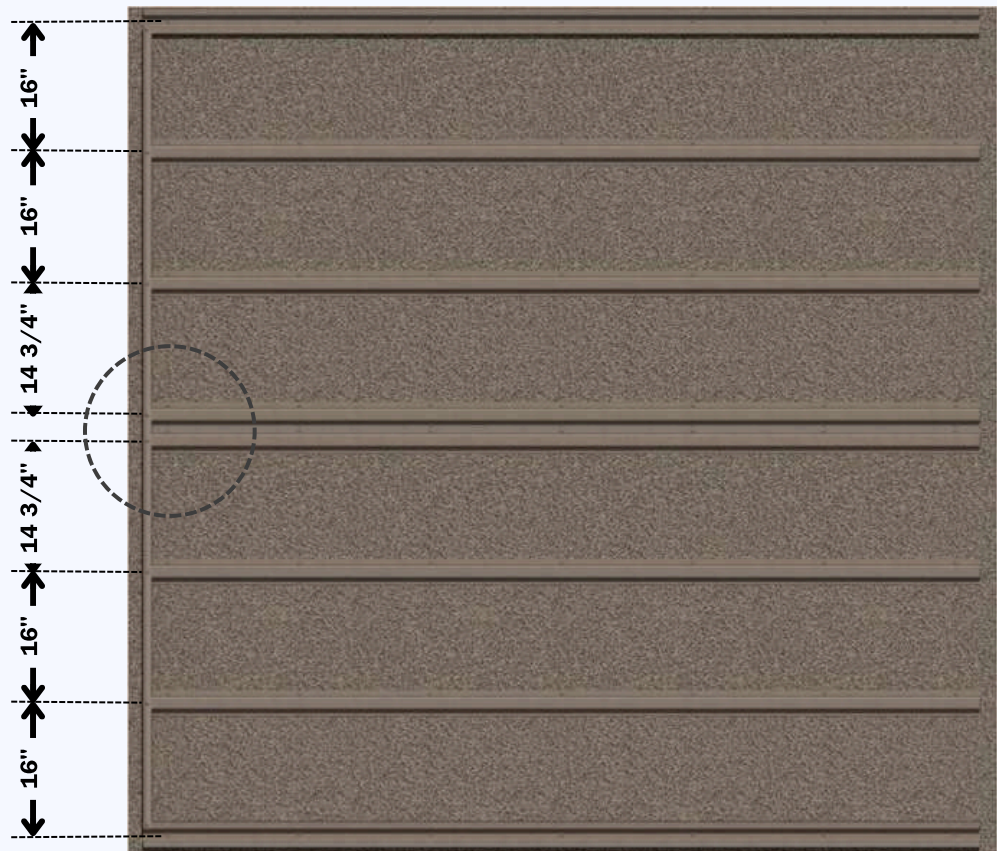
FRONT ELEVATION Siding 6" & 4" Quik-Trim System
